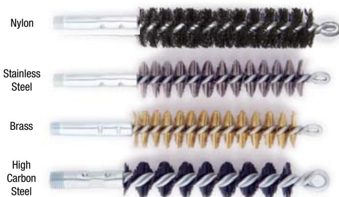
Mill-Rose offers a complete line of condenser tube and heat exchanger brushes available in four bristle materials: High Carbon Steel, Stainless Steel, Brass and Nylon. Bristle sizes are graduated from .008" on small diameter brushes, to .010" on larger sizes to provide consistent cleaning power.
